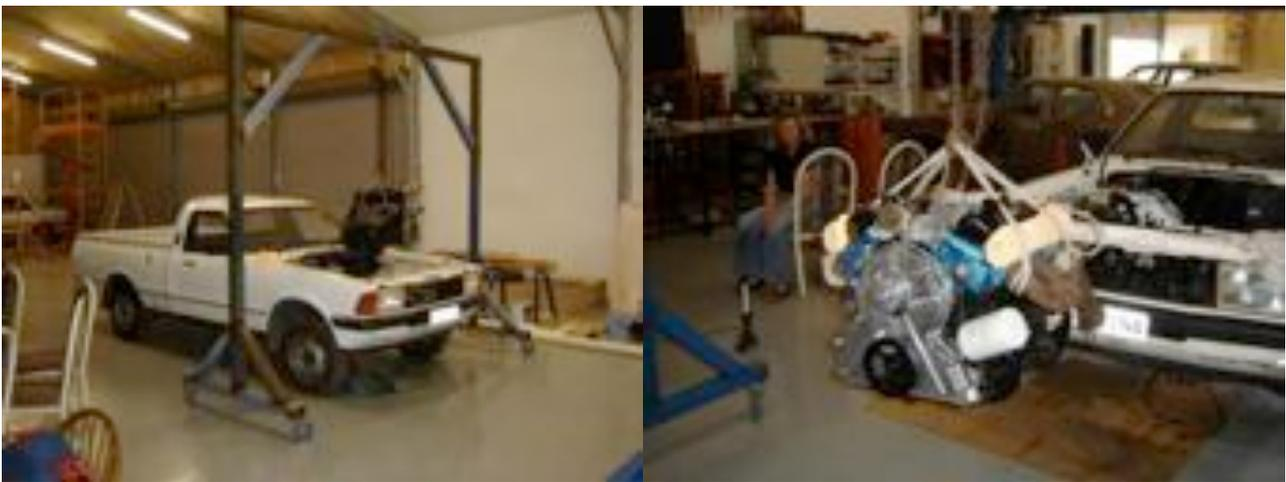
The bottom end was replaced with a rebuilt unit that was sourced from the UK back in 2008. A set of heads rebuilt for unleaded were also fitted along with numerous other new parts.
