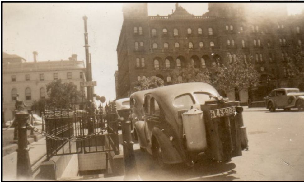
A car in Melbourne outside an underground toilet, fitted with a rear mounted gas producer
